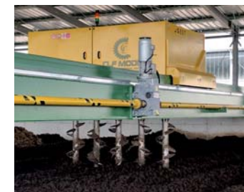
CLF MODIL - MIXING OF THE SOIL IMPROVER AFTER COMPLETION
